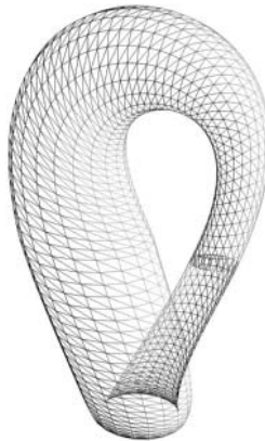
Fig. 12.6. A wire-frame visualization of dataset K, an immersed triangulated Klein bottle with 4000 triangles.
