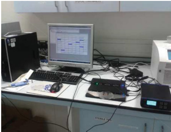
Figure 21.14: The multi-electrode array apparatus connected to a computer monitor. Note the spike trains on the computer screen, these indicate that some of the neurons are firing.
