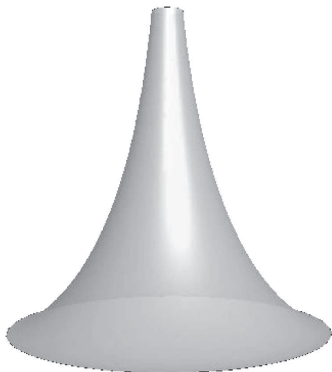
[2.6] The pseudosphere of base radius R has constant negative curvature \mathcal{K} = -(1/R^2) .
