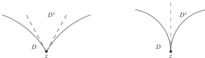
Fig. 10.3 The domain on the left-hand side enjoys the cone property at z , the one on the right-hand side doesn't
