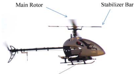
Figure 8.1-6 Helicopter main rotor with a stabilizer bar.
