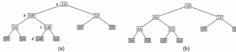
Figure 21.13: A tournament tree before and after inserting an item of size 0.45.
