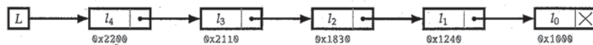
Figure 7.7: The reversed list for the list in Figure 7.6(a). Note that no new nodes have been allocated.
